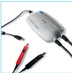
Developed specifically for the automotive industry, AVL DiTEST HV Safety 2000 – the high-voltage measurement module – guarantees stringent compliance with all safety requirements and the safety in the workshop. AVL DiTEST HV Safety 200 is the first “all in one” device able to perform measurements according to UNECE R100. It supports the requirements of a measurement with 1 ampere and this exclusively using the standard USB port, without any additional power supply or batteries.
