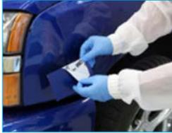
3M™ Color Match film is a small adhesive film that makes it easier for painters to choose quickly between different colours by eliminating any risk of error. It is adhesive and easy to re-position, like a Post-it, on all surfaces. It allows users to check the colour being able to observe it from different angles.
